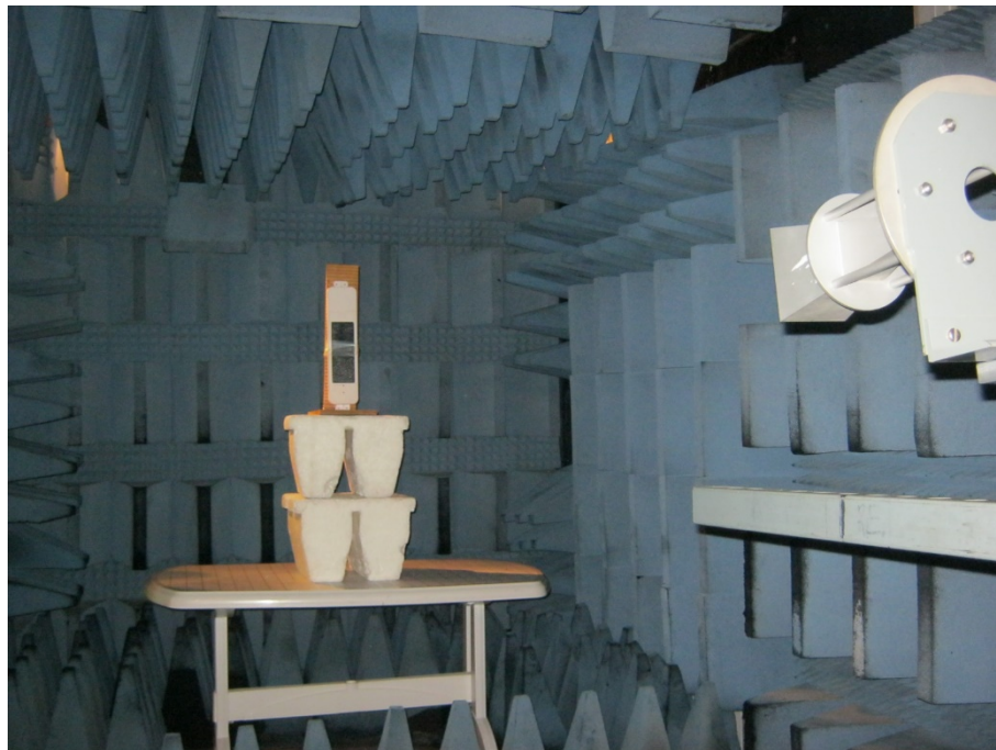
Figure 10. Radiated Emission Test, 18-26.5GHz
