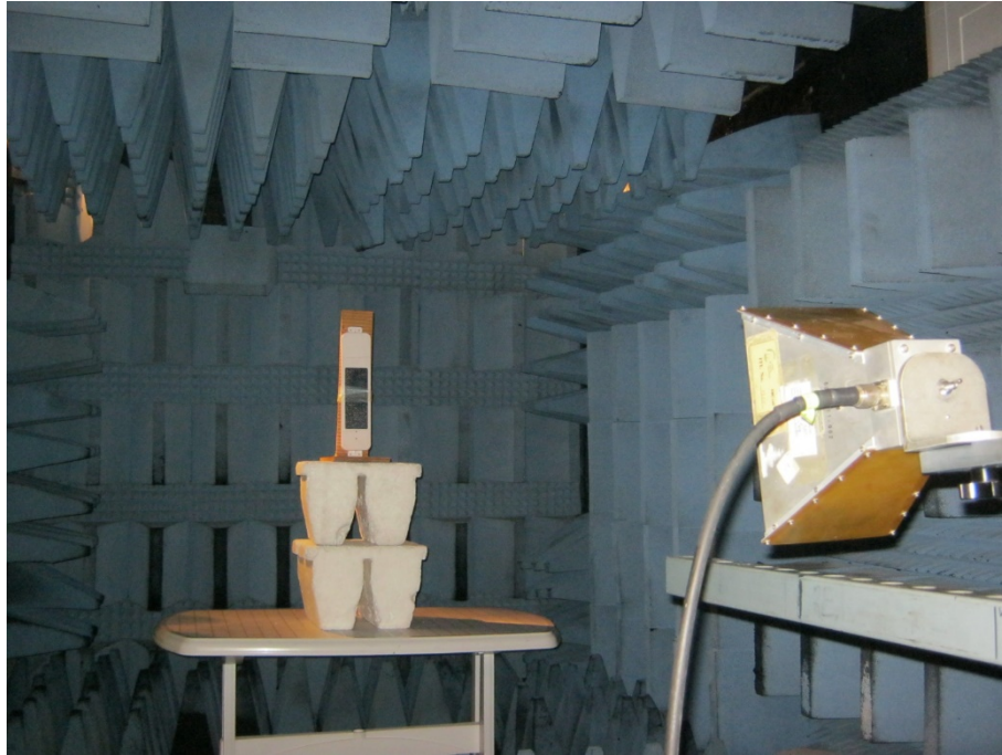
Figure 9. Radiated Emission Test, 1-18GHz and Intermodulation Radiated Emission Test
