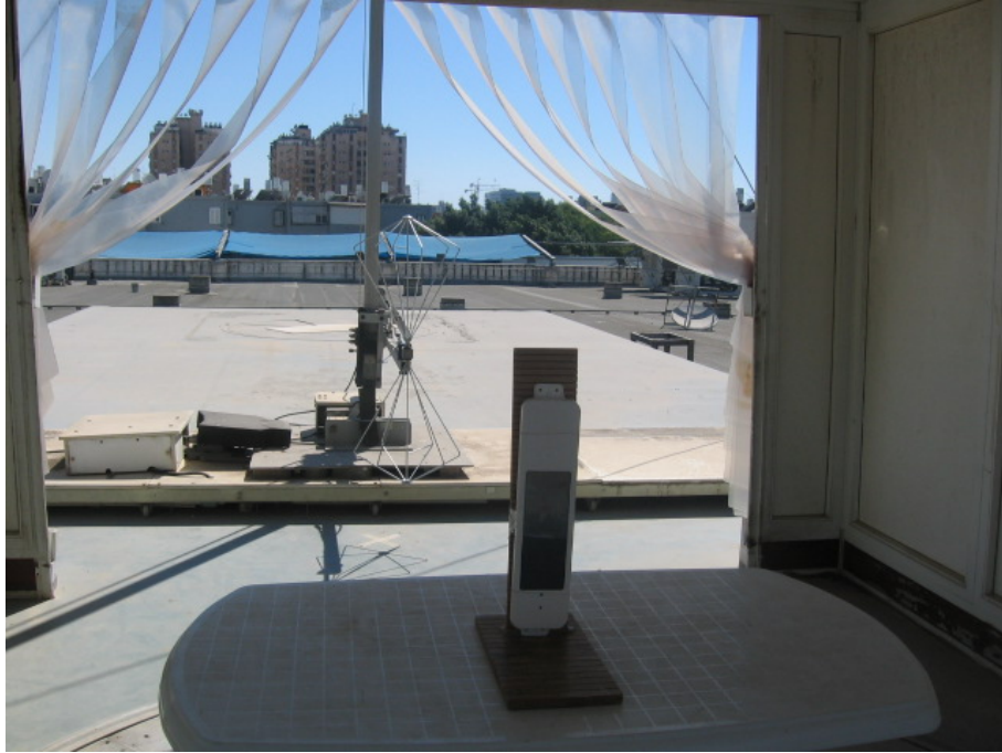
Figure 7. Radiated Emission Test, 30-200MHz
