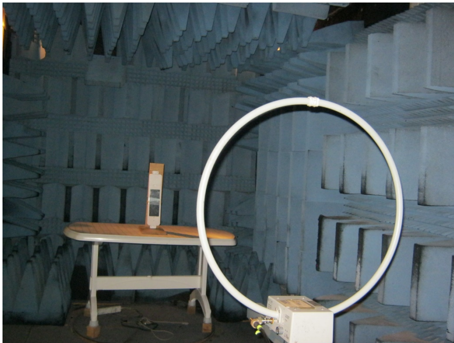
Figure 6. Radiated Emission Test, 0.009-30MHz
